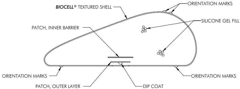
NATRELLE® 410 Breast Implants incorporate orientation marks on the anterior and posterior sides of the shell surface to assist in aligning the implant vertically in the pocket. Two orientation marks are present on the anterior side of the implant in the lower pole. Depending on the style, there will be either 3 or 4 orientation marks on the posterior surface of the implant.
